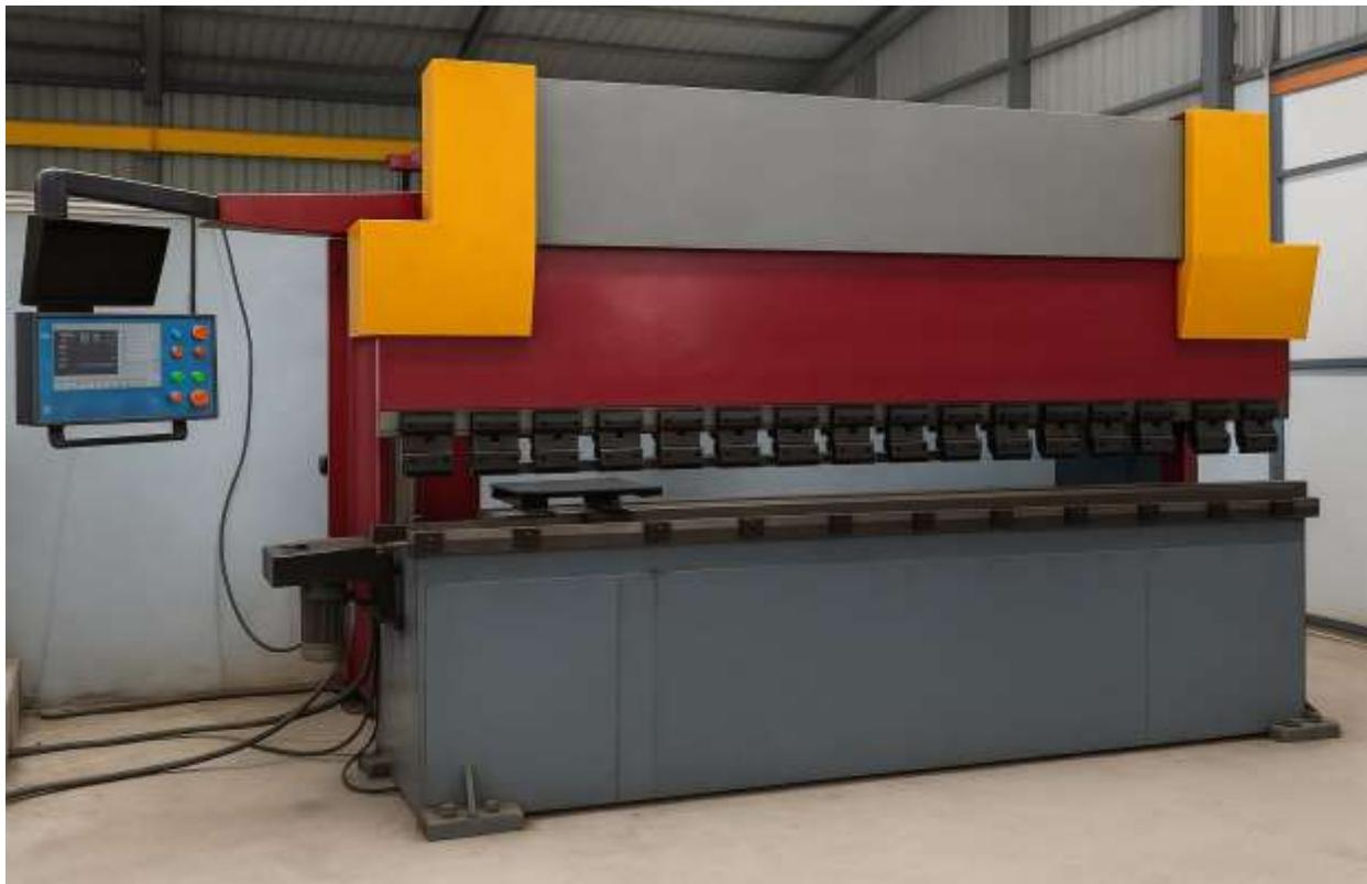
This CNC bending machine from Haco has a width of 3 meters and can bend material thicknesses ranging from 0.5 millimeters to 10 millimeters. It also has a pressing force of 180 tons. Additionally, the machine features an auto-alignment function that automatically corrects the bending angle if any draft or deviation occurs, ensuring precise and accurate bends every time.
