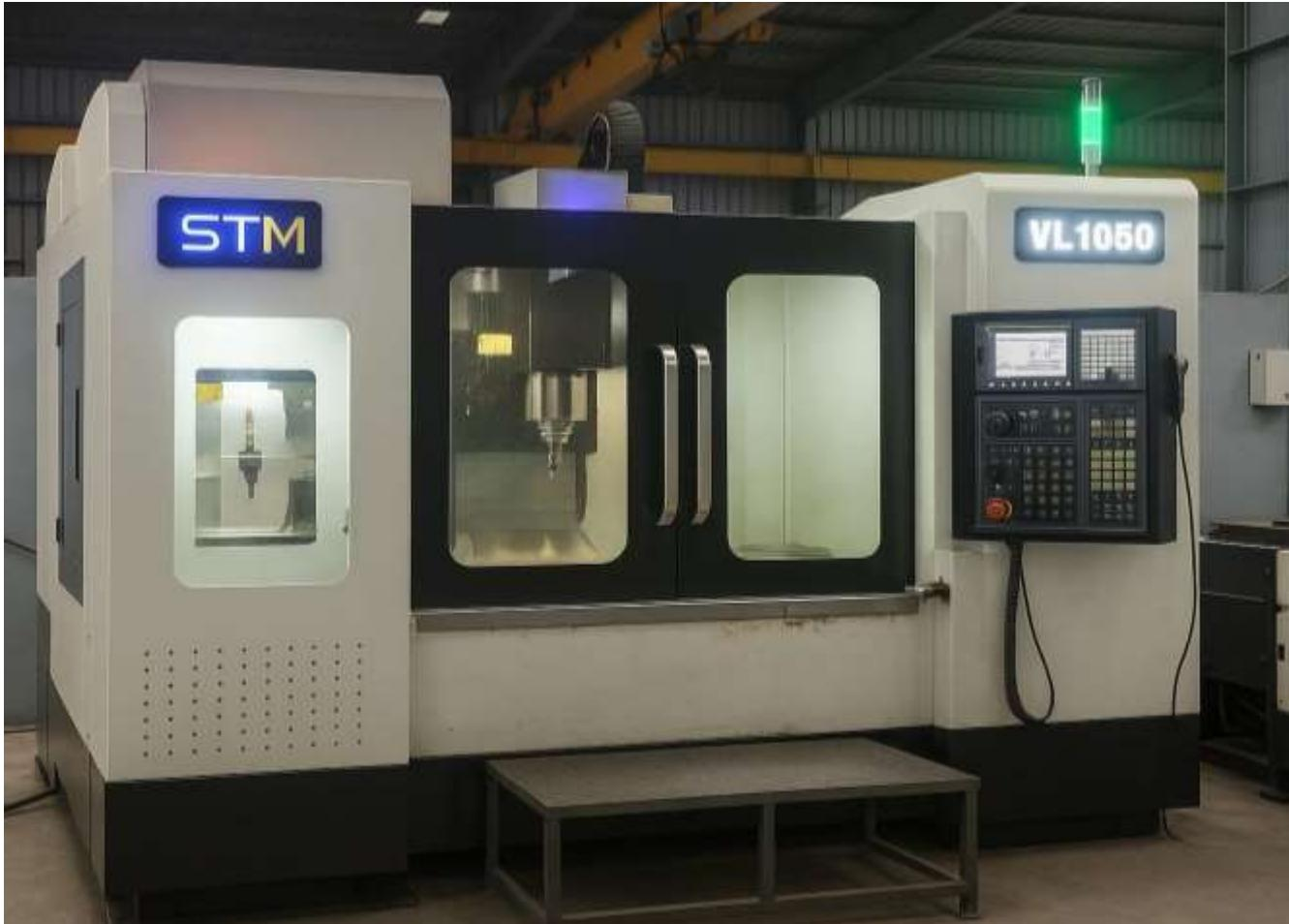
This Vertical Machining Center (VMC) features travel dimensions of 1000 mm in the X-axis, 1000 mm in the Y-axis, and 500 mm in the Z-axis. It is equipped with a Mitsubishi M80 control system and a 24-tool Automatic Tool Changer (ATC), making it highly efficient and versatile. This machine was acquired one year ago and has been an integral part of our operations.
