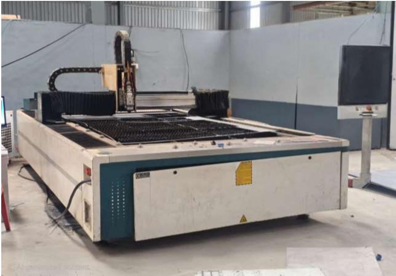
This is a 1.5 kW fiber laser cutting machine, capable of cutting a variety of metals such as stainless steel, mild steel, aluminum, and brass. The cutting capacity typically depends on the thickness of the metal, but in this range, it can easily cut metal sheets up to around 10 millimeters.
